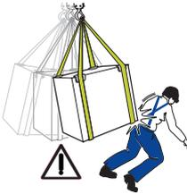
Transport of the equipment, especially by road, must be carried out by suitable ways and means for protecting the components (particularly electronic components) from violent shocks, humidity, vibrations, etc. **During handling, do not make any sudden or fast movements that could generate dangerous swinging.**
