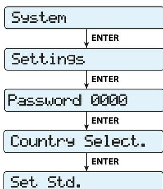
3. After having reset the timer, it will be possible to change the grid standard with the one required in the menu SYSTEM > SETTINGS > Country Select. > Set Std.
