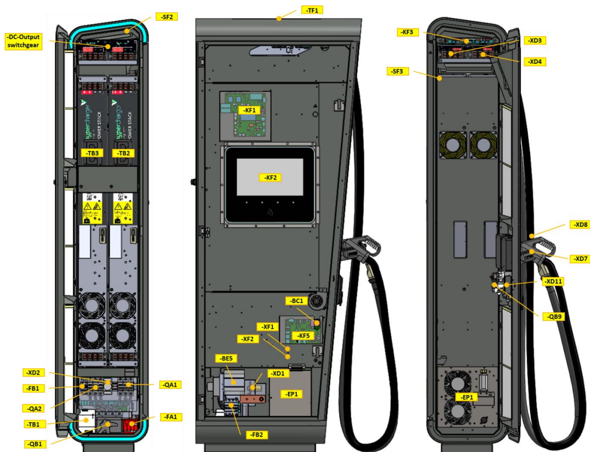
Figure 14: Internal view hypercharger HYC200 (service-, display-, charging cable side)
