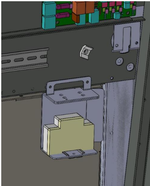
Figure 30: Location of the contactors in the hypercharger
