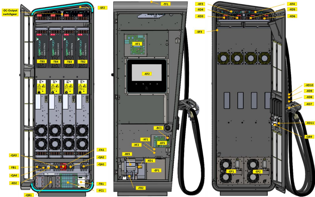
Figure 15: Internal view hypercharger HYC400 (service-, display- and charging cable-side)
