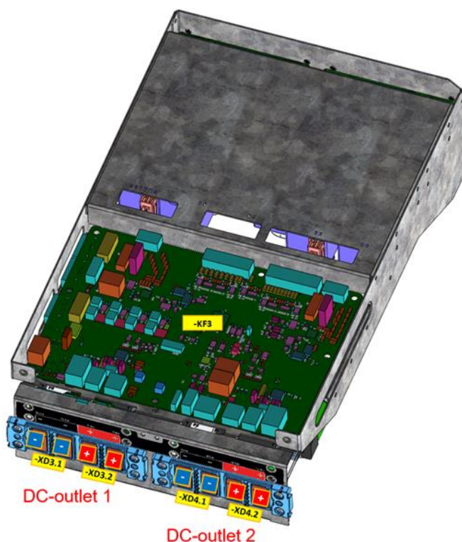
Figure 22: DC output switchgear of the HYC200 (top view)
